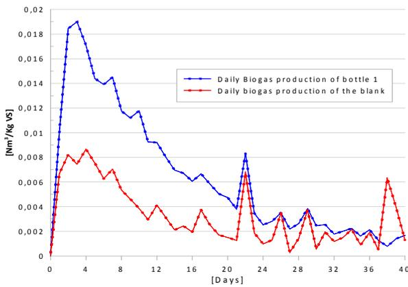
Fig.3. Daily biogas production of the two bio-reactors
