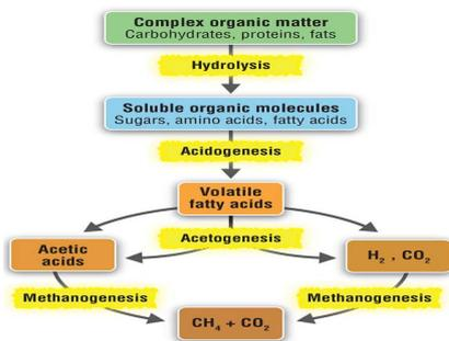
Fig.1. Different steps of anaerobic digestion process
