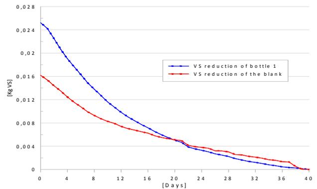
Fig.5. (VS) reduction of the bio-reactors during the biogas production
