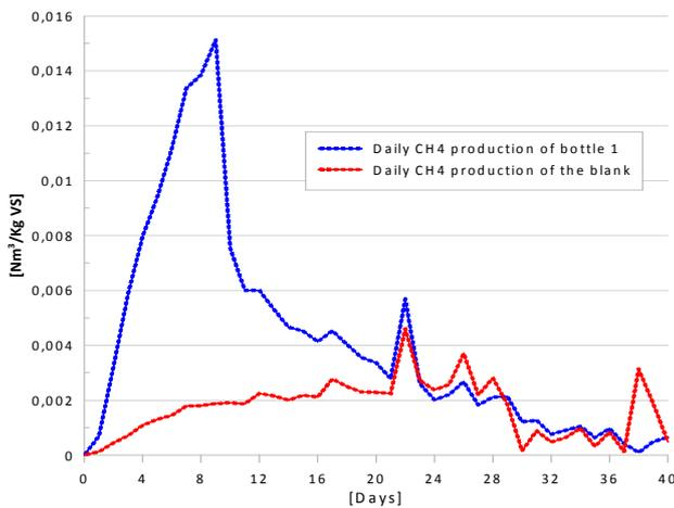
Fig.4. Daily CH<sub>4</sub> production of the two bio-reactors
